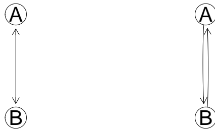
Figure 3: rEG laid out with recipEdges set to combined (left) and distinct (right).
