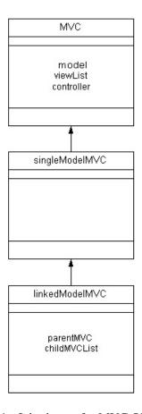
Figure 1: Inheritance for MVC Objects.
