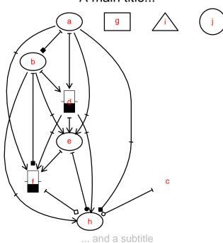
There is also the option to pass a user-defined function as arrowhead or arrowtail parameter to gain even more control. Similar to node shapes, the function has to be able to deal with several parameters: The first parameter gives the center of the location of the arrowhead or tail. The additional parameters col, lwd and lty are color and line styles defined for the edges.
